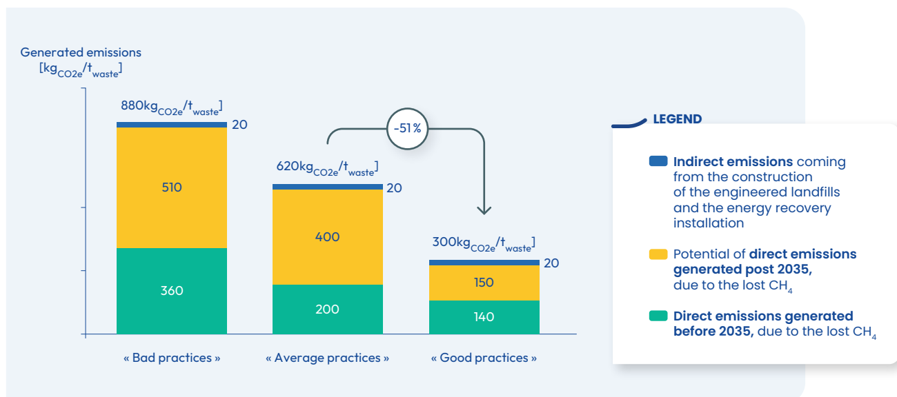
FIGURE 10 Comparative analysis illustrating emissions from landfills with “poor”, “average” and “good” operating practices, based on European data
