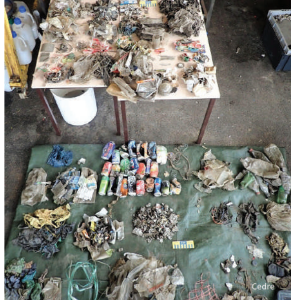
Figure 22: Characterisation of waste in stormwater discharge (Cedre)
