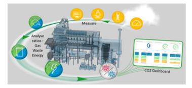
From flue gas to waste composition... by measuring the origin of CO<sub>2</sub> (14C analysis)
