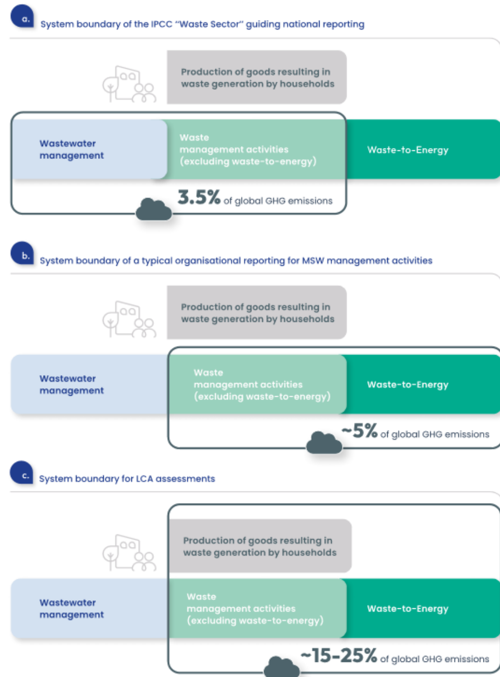
FIGURE 1 GHG emissions from the waste sector depending on the chosen system boundary 3
