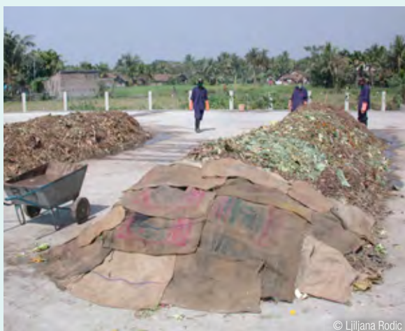
Simple but effective windrow composting, India.
